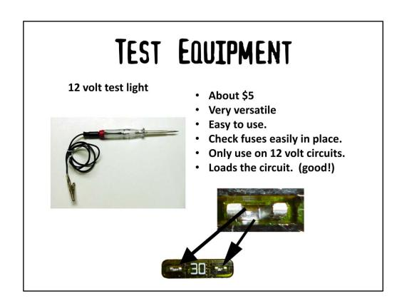
You can use a DVM to make this kind of measurement, but the test light is a quicker and easier way to identify a bad fuse. Not having to pull the fuse out is worth the price!
