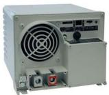
The full 750 watts requires a lot of current, about 73 amps. This is actually quite hard on the batteries. Running in the Boost mode is clearly beyond the battery design limit. Running the vehicle while using the inverter can help.
