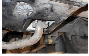
Disconnect the U-bolt holding the pipe on the side of the vehicle and then remove the pipe. A
