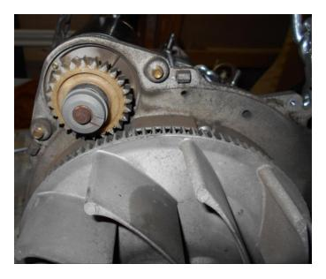
There is a foam gasket between the blower housing and the baffle which had disintegrated. I found material at Lowes which was a good match.
