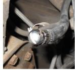
loosen the clamp the hose will pull off, but they often "glue" themselves to the pipe. If it is stubborn, I use an open end wrench the size of the tubing to push on the hose. A little gentle persuasion will do the trick without breaking something. I used a ¼ 20 bolt as a plug.
