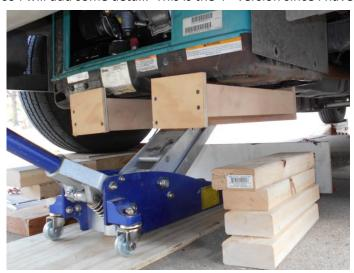
holding the generator with 4 bolts removed.
