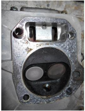
Carburetor and valve cover removed. A new valve cover gasket is a given. The crankcase breather has been removed. These were at about 0.004 inch and the spec is 0.002. Not sure how much real difference that makes.
