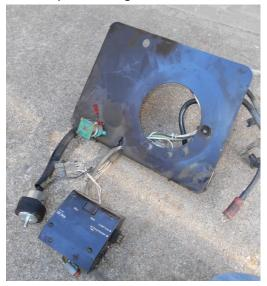
Muffler removed. The bracket which holds the muffler has keyhole slots to make it easier to remove. Note the bonding strap between the engine block and the base.
