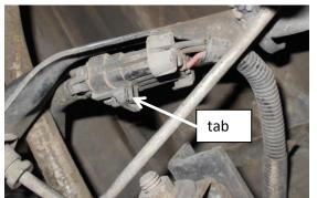
Next disconnect the 12 volt power to the generator. This is a thick cable which is connected directly to the battery, no fuses or protective devices. You did remember to disconnect all the batteries and shore power!
