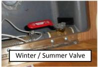
so the water in both tanks will drain out. This valve is located under the bed on the passenger side of the vehicle. In the picture it is shown in the open position or summer mode. This way the two tanks operate as one large tank.
