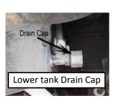
the vehicle below the driver's seat. You can see the cap if you open the gray and black water drain access door.
