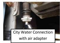
lines, adjust the pressure on your compressor down to 30psi. If you can't adjust the pressure, be very careful not to overpressure the plumbing system. You can do serious damage if the pressure is too high!
