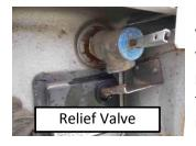
Locate the water heater relief valve behind a panel on the outside of the vehicle. It is shown in the open position in the picture. It is the metal tab with the blue ring. You want this valve in the open position as shown in the picture on the left. This releases any pressure and allows air to enter the
