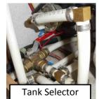
Just below the water pump is the tank selector valve with the red handle. This valve causes the pump to draw water from the inside or the outside fresh water tank. Make sure it is as shown so it draws from the outside tank or summer mode. When in winter mode, it draws from the upper tank. Changing from summer to winter mode requires that you switch both valves correctly.
